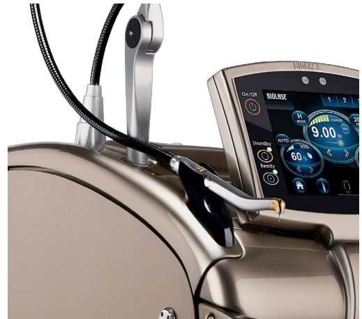
FIGURE 3.3: Handpiece in Handpiece Holder
